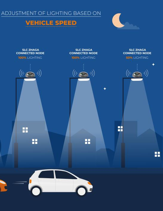
Thanks to its sensors (PIR and radar doppler) and embedded intelligence, the SLS adjusts the light level in real time, based on the presence and
